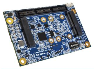
Astro makes use of a high density, board-to-board connector that allows for use with break-out boards.
