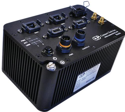
Rosie is designed to meet MIL-STD-810G as well as DO160G for shock and vibration along with ingress protection of IP68.
