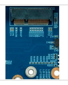
**Note:** Only a M.2 E-Key or M.2 M-Key can be operated at a time. This is a limitation in the amount of available PCIe lanes from the Jetson Module.
