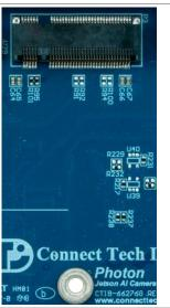
**Note:** Only a USB 2.0 based M.2 3042 B-Key Cellular module can be used with this connector. PCIe is not connected to the M.2 3042 B-Key.
