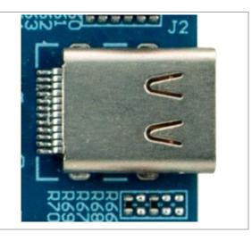
Note 1: This port can be used for host mode access to the NVIDIA® Jetson Nano™ module at 5Gbps only.
