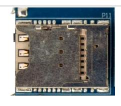
Note: microSD card is on the top, SIM card is on the bottom.
