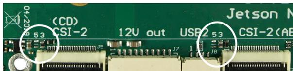
You can find that option near the CSI connector. These components are specially marked with a „3“ and a „5“.
