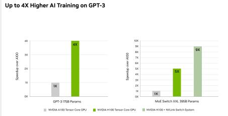
Projected performance subject to change. GPT-3 175B Training A100 cluster: HDR IB network, H100 cluster: NDR IB network | Mixture of Experts (MoE) Training Transformer Switch-XXL variant with 395B parameters on 1T token dataset, A100 cluster: HDR IB network, H100 cluster: NDR IB network with NVLink Switch System where indicated.
