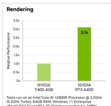
Tests run on an Intel Core i9-12900K Processor @ 3.2GHz (5.2GHz Turbo), 64GB RAM, Windows 11 Enterprise x64, NVIDIA Driver 551.79. Relative speedup for 1080p resolution Arnold render tests. Performance based on prerelease build, subject to change.
